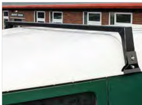
DA5570 Roof bar - single Defender 90 & 110 - 1991 onwards Weight 4kg Load 100kg
