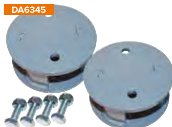
Defender - 90/Discovery 1/Range Rover Classic These 50mm spring spacer blocks are manufactured from 6mm plate with a powder coated finish. The spacers fit between the axle and the spring seats on the front and rear to give you that extra 50mm of lift you need. DA6344 Front pair DA6345 Rear pair
