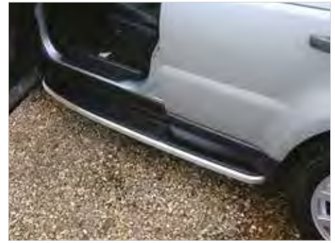
Side Steps VPLSP0040 Side steps with thermo plastic elastomer side step top and brushed aluminium side trim. Pair.
