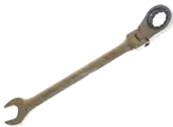
Oil Filter Remover Tool DA1189 For removing and installing oil filters on diesel models of the Freelander 2 and Range Rover Evoque. 27mm combination spanner with flexi head. 400mm long. Manufactured from Chrome Vanadium. Fully polished with ratchet. Manufactured to Ansi standards.
