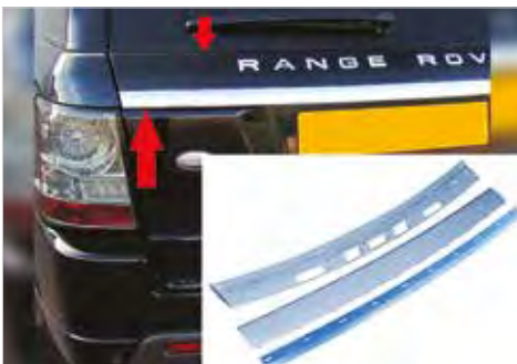
Tailgate Conversion Trim Kit DA6290 Range Rover Sport - 2005 - 2011 The rear tailgate on the Range Rover Sport changed in 2012 from a two piece tailgate (with opening top window section) to a one piece tailgate and above the registration plate a new silver strip was added that went the width of the tailgate. If you have a 2005 - 2011 model and want to make it look like the 2012 model from the rear you can fit this clever conversion kit. The kit consists of 3 panels - 1. Underside base - section made from ABS plastic in grey primer finish - you will need to paint this part black. 2. Top section - supplied in primed ABS plastic ready for painting body colour 3. Strip section - chrome plated plastic. This is a bolt on replacement kit that replaces the existing panels on the upper tailgate. Easy to fit. More details online.
