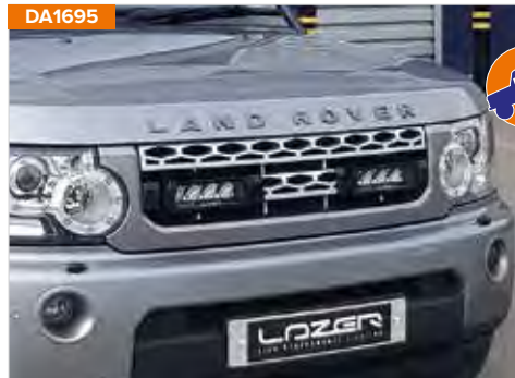
DA1695 NEW Discovery 4 - Up to 2014 Triple-R 750 LED spotlights grille integration kit
