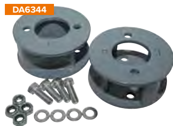
Defender - 90/Discovery 1/Range Rover Classic These 50mm spring spacer blocks are manufactured from 6mm plate with a powder coated finish. The spacers fit between the axle and the spring seats on the front and rear to give you that extra 50mm of lift you need. DA6344 Front pair DA6345 Rear pair
