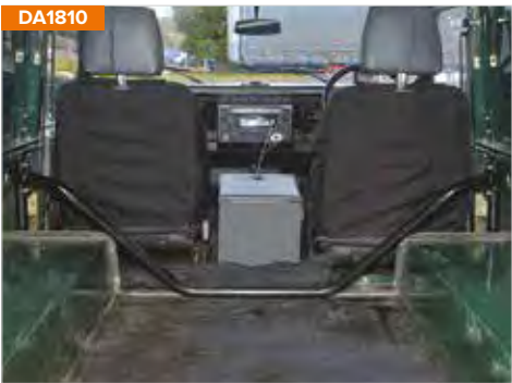
DA1810 Defender OEM bulkhead removal bar kit
