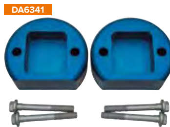
Discovery 2 These 40mm spring spacer blocks are machined from high quality aluminium and anodised deep blue. DA6341 Front pair With this kit you are able to retain the standard springs and shock absorbers. Use in conjunction with DA6342.
