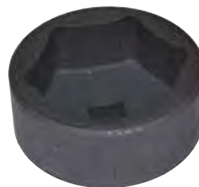
Oil Filter Socket DA1176 36mm oil filter socket - 3/8" drive Designed to protect the corners of the filter from damage. Defender - Puma 2.2 & 2.4 Freelander 1 - Td4 Range Rover L322 - 2002 - 2009 - M57 3.0 diesel & M62 4.4 V8 petrol
