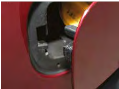
DA1114 Discovery 3/Discovery 4/Range Rover Sport - 2015 - 2013 This handy little OEM kit is used to repair the temperamental fuel latch.
